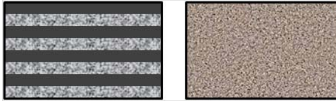
Figure 22. Schematic of possible structures for nanostructured coatings. (Left) multilayered microstructure (e.g., TiN/TiC) for nanocomposite coatings; (right) homogeneous nanostructured coating (e.g., NiCoCrAlY alloy). (Image credit: L. Filipponi, iNANO, Aarhus University, Creative Commons Attribution ShareAlike 3.0).
