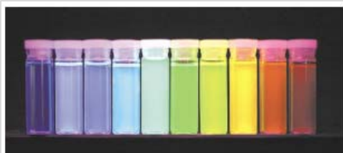
Figure 13. Ten distinguishable emission colours of ZnS-capped CdSe QDs excited with a near-UV lamp. From left to right (blue to red), the emission maxima are located at 443, 473, 481, 500, 518, 543, 565, 587, 610, and 655 nm. (Reprinted by permission from Macmillan Publishers from Macmillan Publishers Ltd: Nature Biotech. (2001) 19, 631-635, Copyright 2001).
